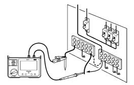
Ex. Checking the continuity of ground wiring
