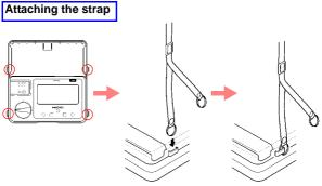
Pass the ring on both ends of the supplied strap through each of the four holes in the instrument.
