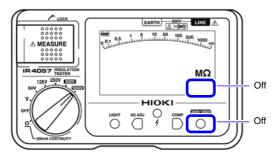
The instrument will return to the state described in Step **1**. when 1 minute elapses after the last measurement or operation. Press
